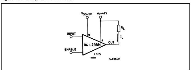
Note: For INPUT Switching, set EN = H For ENABLE Switching, set IN = L
