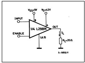
Note: For INPUT Switching, set EN = H For ENABLE Switching, set IN = H
